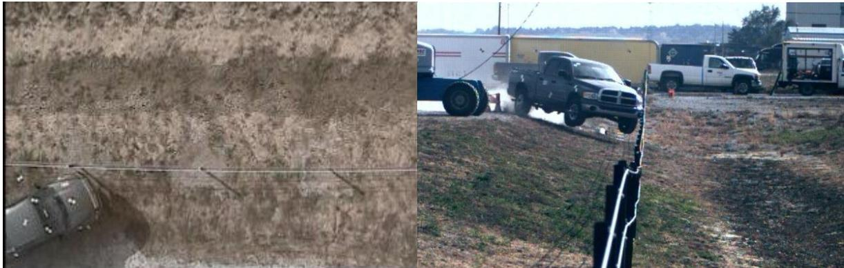
**Figure 3.1** Vehicle-Cable Impact of Test 4CMB-1
